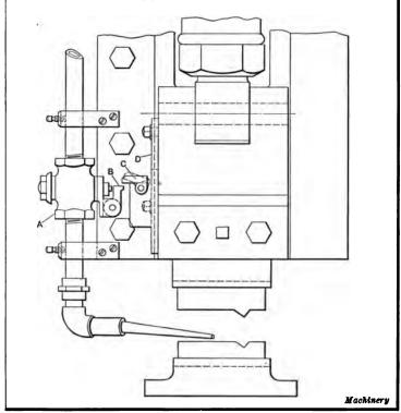
Fig. 16. Pneumatic Press Attachment for Automatically Removing Work
